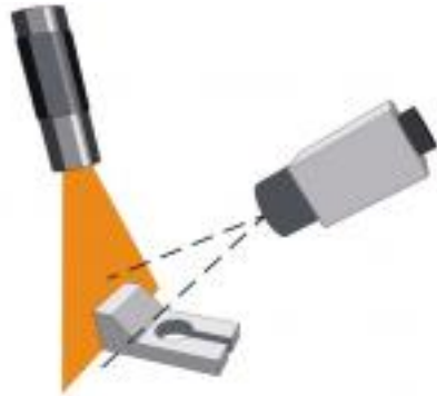
The 3D shape of an object is determined by measuring the profile of the object along a projected line of light.
